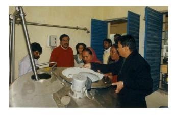
With the increase in milk production, need for creation of infrastructure was felt. A bulk cooler of 500 lit per day capacity was installed. This bulk cooler will save the farmers of remote villages to transport the milk to the milk union chilling plant. This would save the time as well as chances of spoilage of milk. One such unit would
